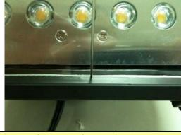
Test for protection against access to hazardous parts
