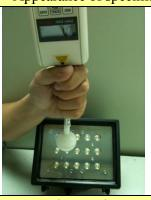
Test for protection against access to hazardous parts
